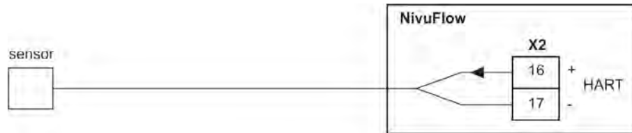
Fig. 16-5 Connection of 2-wire sensor for level measurement
