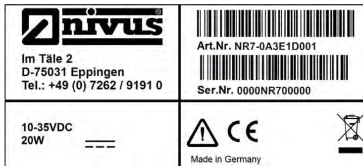
Fig. 9-6 Nameplate DC version
