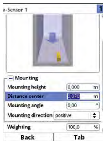
Fig. 23-20 Entering sensor positions related to application centre
