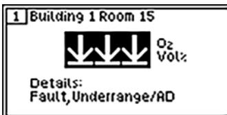
Here, the sensor signal in the transmitter has even fallen below the measuring range of the transmitter electronics. It is possible that a gas with a negative cross-sensitivity is present at the measuring point or that the Zero point signal has drifted away due to aging of the sensor or due to environmental influences.
