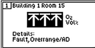
In this case the sensor signal in the transmitter has exceeded the measuring range of the transmitter electronics. The cause could be a very high gas concentration at the transmitter or a gas with a very high cross-sensitivity. It is also possible that the sensor or the transmitter electronics are defective.
