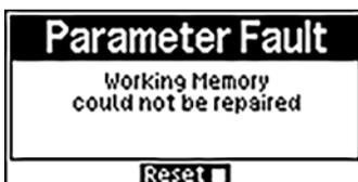
There is incorrect data stored in the parameters in the RAM, which cannot be corrected automatically due to a hardware defect on the mainboard.
