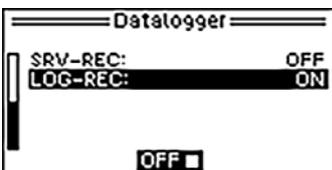
The data recording on the microSD card for service purposes can be started for a maximum of 8 hours in the SRV-REC menu item. The recording can also be stopped manually here again.
