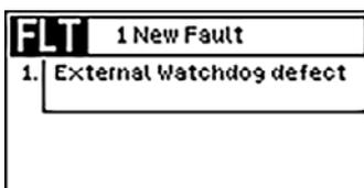
A malfunction was detected when checking the external monitoring module on the mainboard.
