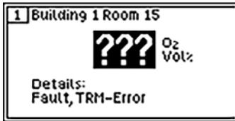
In this case, there is a malfunction of the digital transmitter. It is possible that the supply voltage of the transmitter is too low or too high or the transmitter itself is defective.
