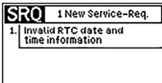
Date and time are invalid in the clock module of the GMA200. This indicates that the buffer battery of the clock module is empty or not properly contacted, so that when the GMA200 is switched off, the clock module cannot continue to operate and thus the date and time are lost.
