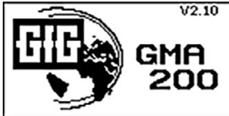
At system start the GfG logo, the device name and first the version number of the bootloader and then the version number of the mainboard firmware is displayed. During this time, various internal self-tests are performed. After completion of the internal tests, a short test of the display, all LEDs and the horn is performed. During the entire time, the yellow "FLT/GMA" fault LED is lit and the relays are de-energized.
