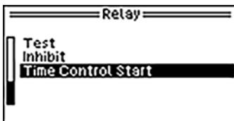
The GMA200 offers the possibility to switch relays time-controlled. If such a time control has been configured and set as a start condition in the service menu using the GMA200Config software, it can be started here.
