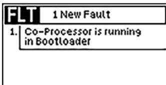
After a reboot the slave processor on the display board only runs in the bootloader because the program of the slave processor is faulty.
