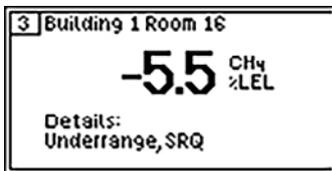
At the transmitter, the signal zero point has drifted away negatively, so that the measuring range of the transmitter has been clearly undercut (Underrange typically < -5 % from measuring range).
