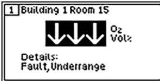
In this case the sensor signal in the transmitter has clearly fallen below the transmitter measuring range (usually < -7.5 %). It is possible that a gas with a negative cross-sensitivity is present at the measuring point or that the Zero point signal has drifted away due to aging of the sensor or due to environmental influences.
