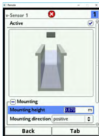
Fig. 23-16 Setting the mounting height
