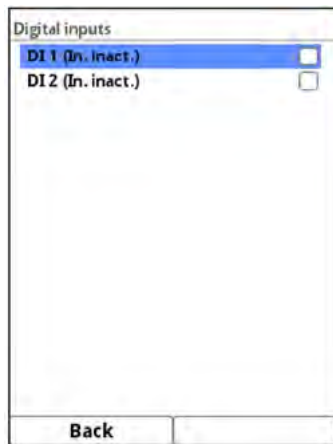
Fig. 42-4 Indication of digital inputs
