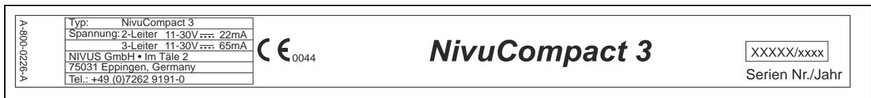
**Fig. 3-1 Nameplate of NivuCompact 3 without Ex approval**
