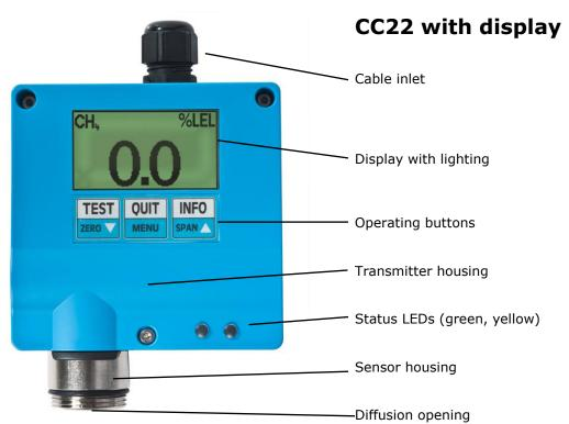
The gas sensor and the transmitter electronics are installed in the transmitter housing. The electronics convert the measurement signal into a gas concentration and indicates it with an analogue current signal of 4-20mA or 0.2-1mA or with a digital RS485 bus signal in the Modbus RTU protocol. The gas concentration and the status information are displayed on the display version.
