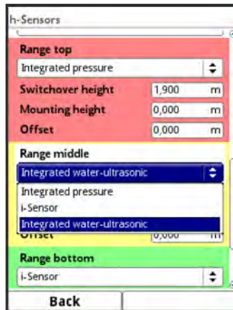
Fig. 39-16 Assignment Level Sensor to Parameterisation Range
