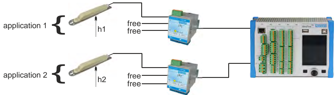
Fig. 25-5 Pressure cell for level measurement
