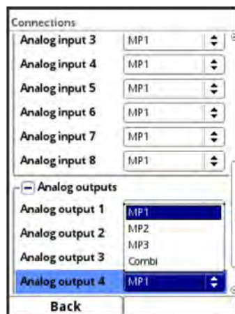
Fig. 45-5 Assigning Inputs/Outputs to the Combi Measurement Place
