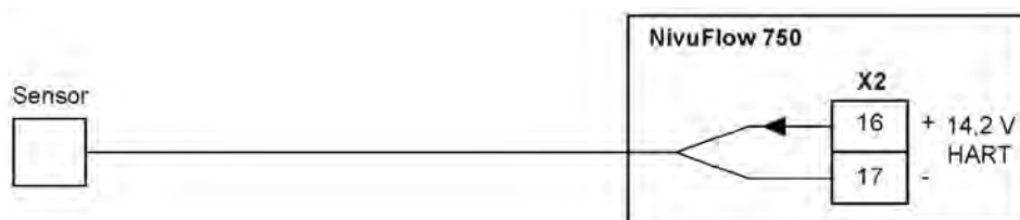
Fig. 23-15 Connection of 2-wire sensor for level measurement
