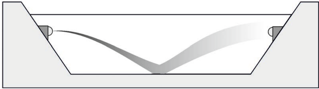
Fig. 9-4 Extreme vertical density difference due to salinity (principle)
