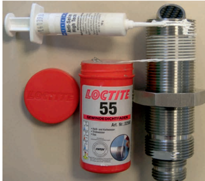
Fig. 10-56 Mounting preparation screw-in sensor
