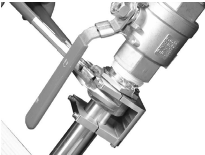
Fig. 10-37 Loosening the sleeve nut for sensor dismantling
