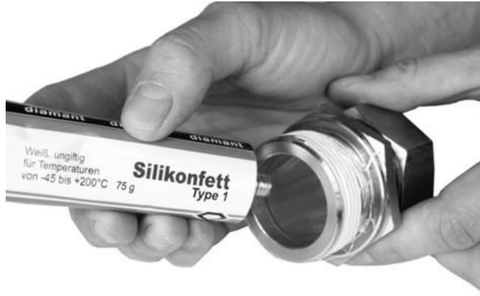
Fig. 10-30 Greasing the sensor screw connection
