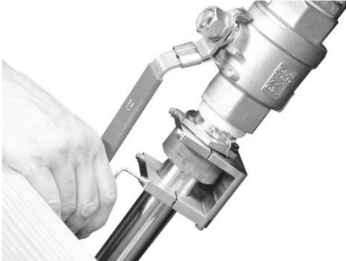
Fig. 10-36 Fastening the final clamping element
