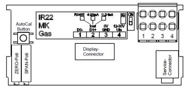
For digital data transfer via RS485 the bus cabling is depending on different factors. This includes the composition of the bus as a strand or ring, the number of transmitters on the bus, the distance of the individual transmitters from the GMA, the transmitter type / model, the sensor type and, of course, from the bus cable type. It is necessary to check in the individual case, if the
