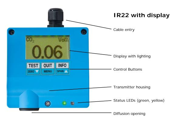
The gas sensor and the transmitter electronic are built-in the transmitter housing. The electronic transforms the measuring signal in a gas concentration and signalises it with an analogous current signal from 4-20mA or from 0.2-1mA or a digital RS485 bus signal in the Modbus RTU protocol. For the display model, gas concentrations and status information are displayed.
