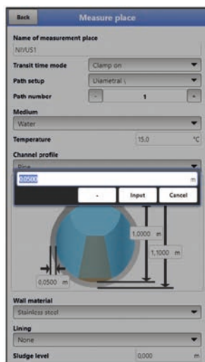
Fig. 34-2 Entering the pipe data
