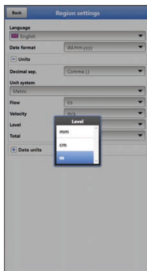
Fig. 42-4 Setting the measurement units
