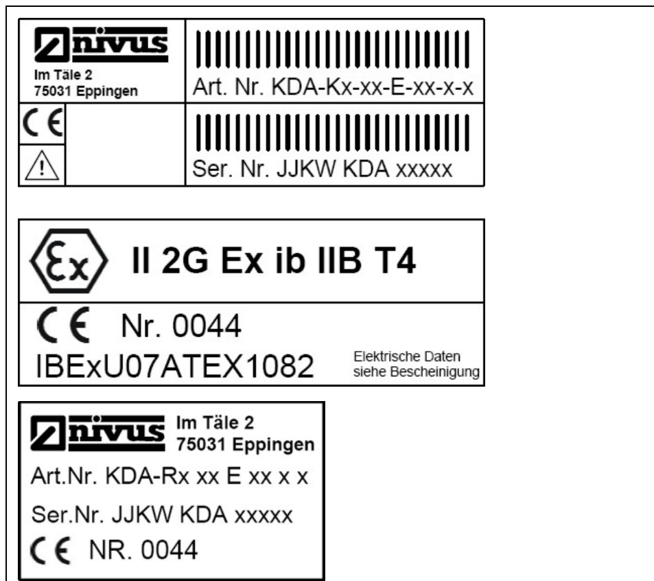
Fig. 3-1 Nameplate flow velocity sensor wedge and pipe
