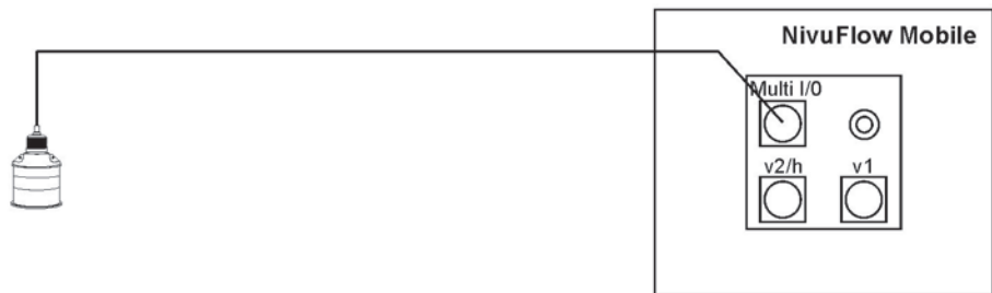
Fig. 25-3 Connection of i-Series and NivuBar Plus level sensors
