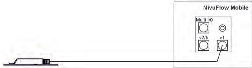
Fig. 25-1 Connection of CSM, CSP and NPP flow velocity sensors
