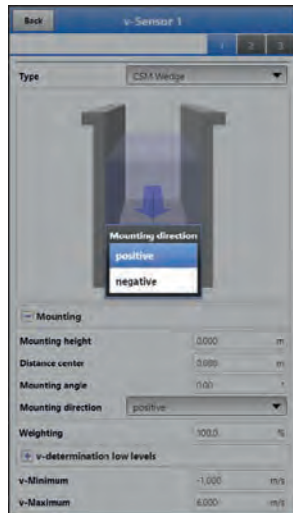
Fig. 39-19 Option to change the Sensor Mounting Direction
